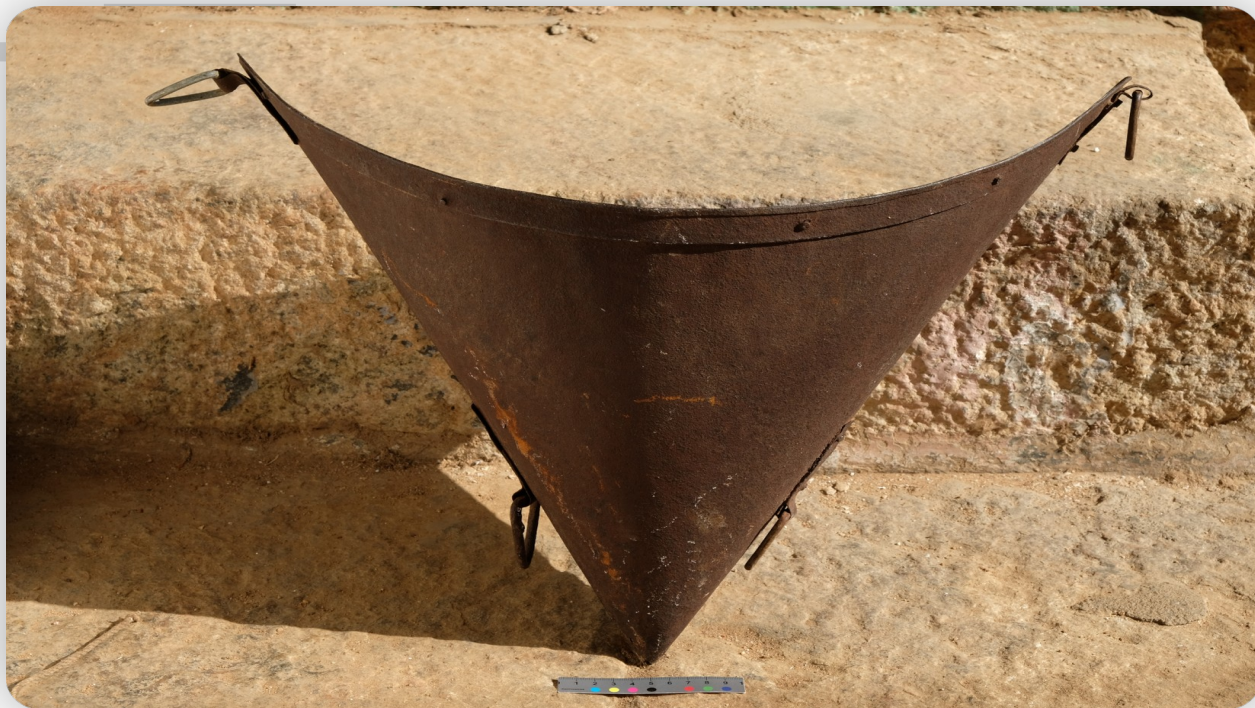
Eravatti - Measuring instrument for running water for Irrigation
